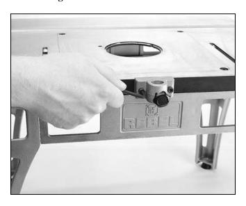
Figure 6. Mounting safety guard bracket.
